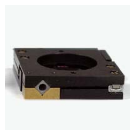
Piezzo Motor Attocube ANT200 Translation table Travel: 0-5mm Resolution: 10nm
